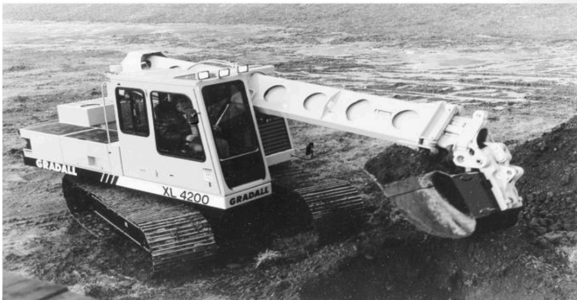
FIGURE 3-4. Telescoping-boom hydraulic excavator. (Courtesy of JLG Industries, Inc.)
