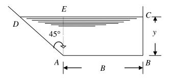
The trapezoidal section *ABCD* is made up of a rectangular portion *ABCE* of dimensions (*B* x y) and a triangular portion *AED* right – angled at *E*. From triangle *AED*, tan  $45^\circ = \frac{ED}{AE} = \frac{ED}{y} = 1$ Hence, ED = y Hence, area of triangular portion =  $\frac{1}{2} x ED x AE = \frac{1}{2} x y x y = \frac{y^2}{2}$ Area of rectangular portion = ByHence, area of trapezoidal section,  $A = By + \frac{y^2}{2}$
