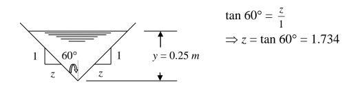
$Q = 80 \ dm^3 \ s^{-1} = 80 \ x \ (10^{-1})^3 = 80 \ x \ 10^{-3} \ m^3 \ s^{-1}$ (*Note:* 1  $\ dm = 10 \ cm = 0.1 \ m = 10^{-1} \ m$ ) Wetted area of channel section,  $A = Zy^2 = 1.734 \ x \ (0.25)^2 = 0.108 \ m^2$ As per the continuity principle, we have, Topic: Flow in Open Channels (Uniform Flow)
