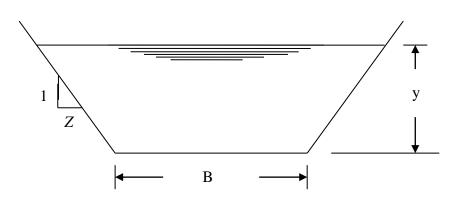
Side slope of channel section = 1 vertical : *z* horizontal = 1 : 1.5 Let the bottom width of channel section be *B* and the depth of flow be *y*.  $Q = 2.7 \ m^3/s$ C = 44.5Bed slope S = 1 in  $4000 = \frac{1}{4000} = 0.00025$ B = ?y = ?
