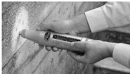
Figure 4.31. Rebound / Schmidt hammer
