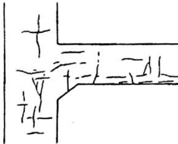
Figure 4.21. Rusting of reinforcing bars
