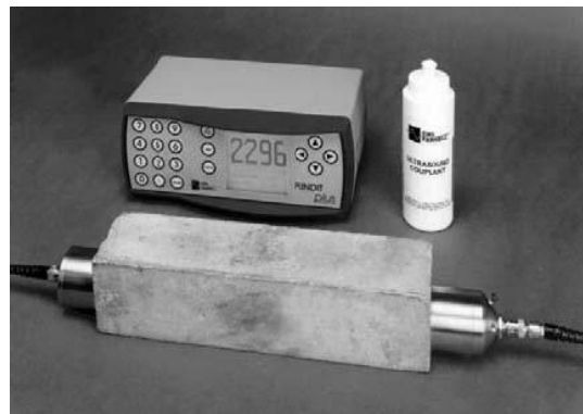
Figure 4.33. Ultrasonic Pulse Velocity Test setup
