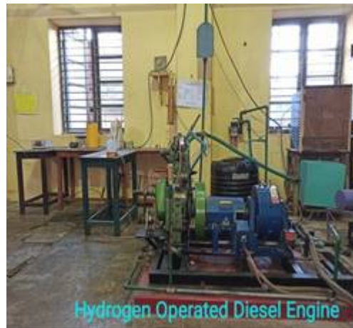
Hydrogen engine test rig
