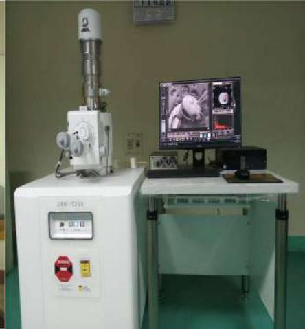
**Scanning Electron Microscope - EDS**
