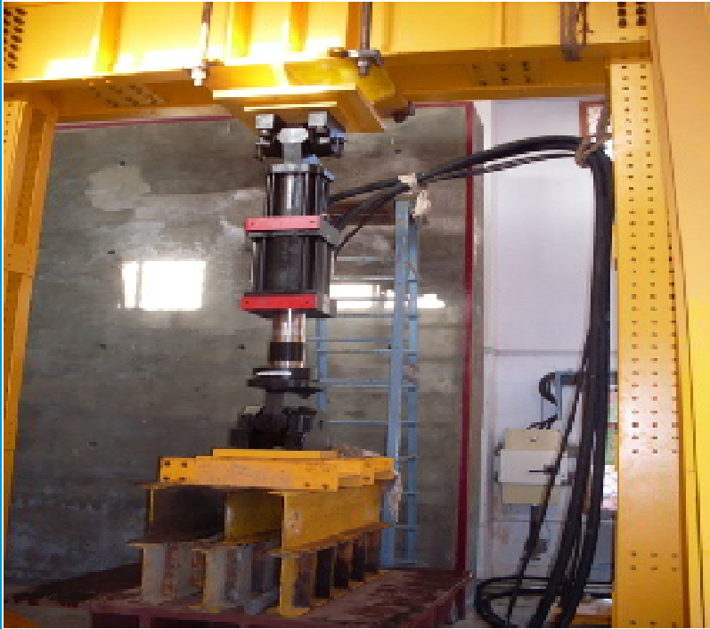
MTS Hydraulic Actuator with Test Frames
